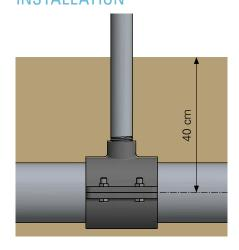
It is recommended to place the distribution pipe in the soil at a depth of at least 40 cm.
