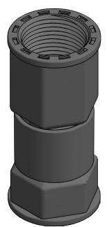
The Fast Sprinkler Coupling is a ¾ inch bayonet type connector. It is the simplest, low-cost solution to connect and disconnect at will a sprinkler to a riser pipe, allowing storage of the sprinklers when not in use.
