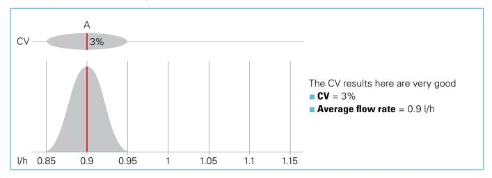
Next to it a second injection molding machine [B] that also produces drippers of a nominal flow rate of 1.0 l/h, and the CV check presents the following results:
