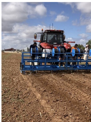
Above: Coils of dripline are mounted on an implement similar to a tyne planter to bury dripline and cover back over with soil
