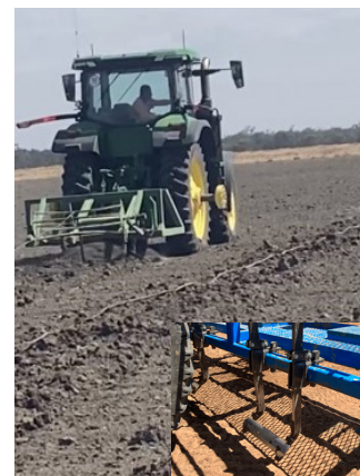
Above: An implement with a blade is used to break dripline out of the soil for it to be recoiled for recycling
