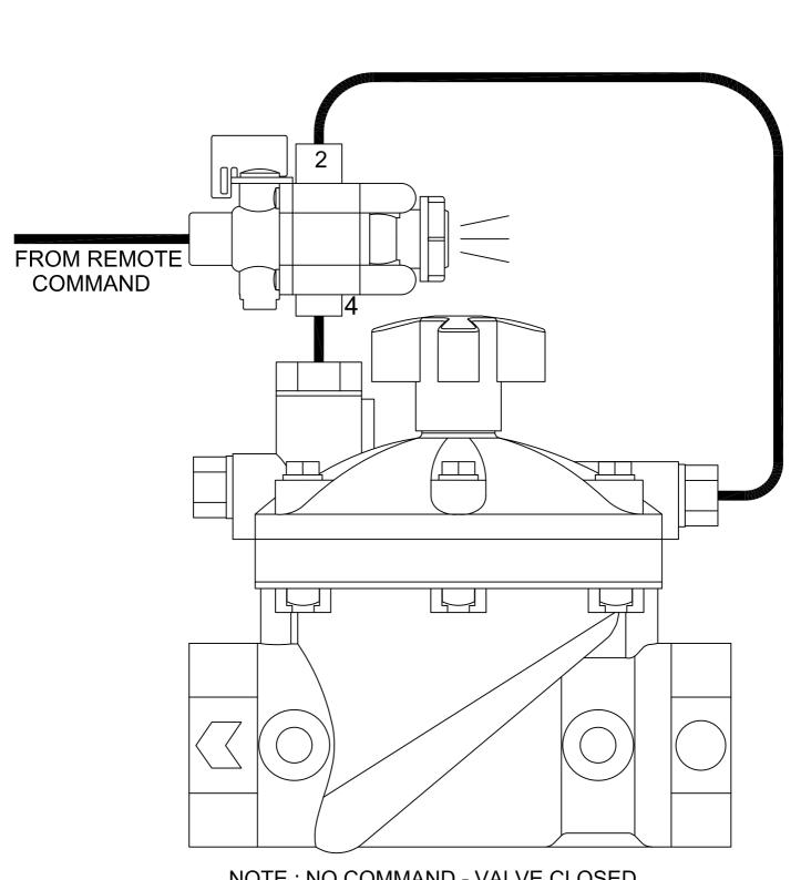
NOTE: NO COMMAND - VALVE CLOSED COMMAND - VALVE OPEN
