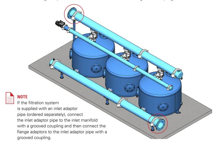
12. Connect the flange adaptor to the backwash flow-control valve with a grooved coupling.
