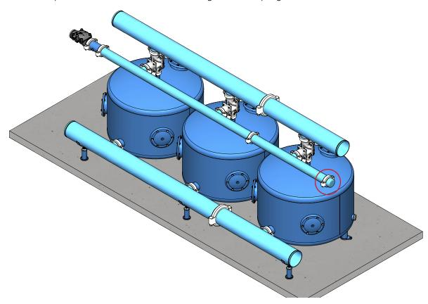
9. Connect the end-cap to the inlet manifold with a grooved coupling. Make sure that the end-cap is placed with the socket for the air valve pointing upwards and the socket for the control assembly pointing sideways.
