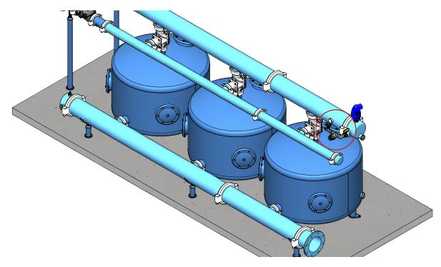
17. Place the stand of the backwash controller so that it is close to the control assembly (make sure it meets your needs for both operation and maintenance). Secure it to the concrete slab with 10 mm spreading anchor bolts.
