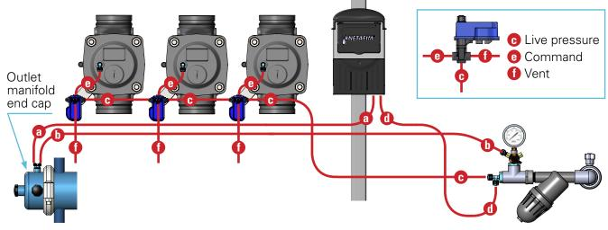
**20.** Connect the solenoids to the BackFlush controller expansion cards in sequence, from left to right. Red wire = + / black wire = common (inversing wire polarity will change NC to NO).
