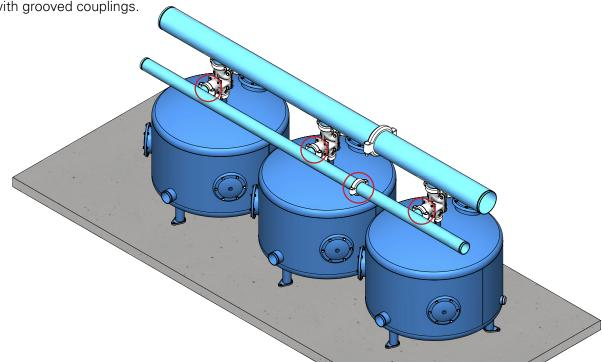
**5.** Connect the outlet manifold to the outlets of the tanks and the outlet manifold sections to each other with grouved couplings
