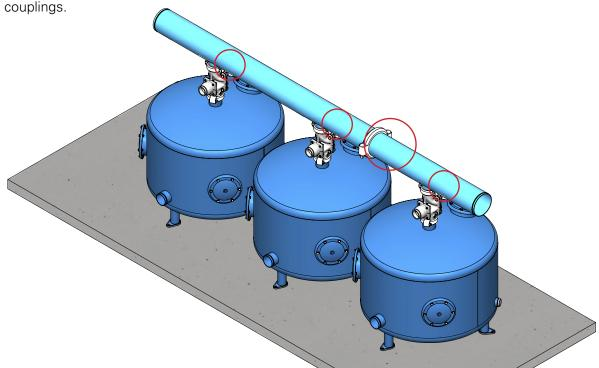
**4.** Connect the backwash manifold to the backwash valves and the backwash manifold sections to each other with grooved couplings.
