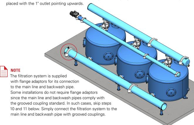
11. Connect the flange adaptors to the inlet and outlet manifolds with grooved couplings.
