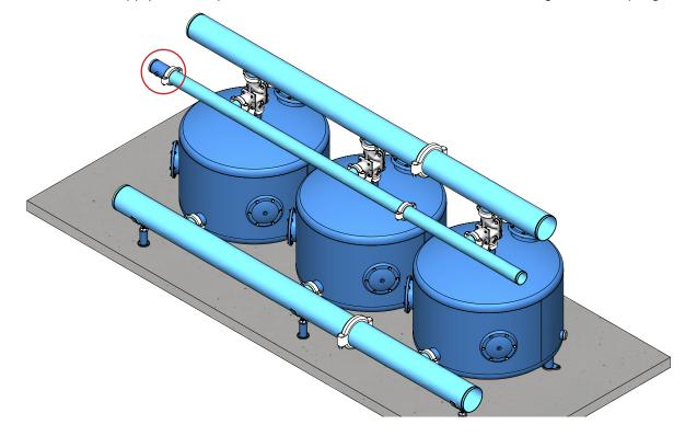
**b.** Connect the backwash flow-control valve to the backwash manifold's short section with a grooved coupling. Be sure that the position of the valve is per the flow arrow marked on the valve.
