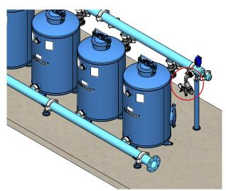
17. Place the stand of the backwash controller so that it is close to the control assembly (make sure it meets your needs for both operation and maintenance). Secure it to the concrete slab with 10 mm spreading anchor bolts (not supplied).
