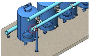
10. Connect the end-cap to the inlet manifold with a grooved coupling. Make sure that the end-cap is placed with the socket for the air valve pointing upwards and the socket for the control assembly pointing sideways.
