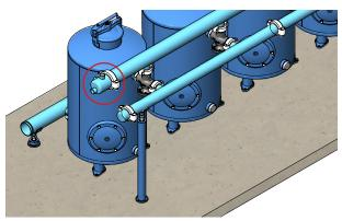
**11.** Connect the end-cap to the outlet manifold with a grooved coupling. Make sure that the endcap is placed with the socket for the air valve pointing upwards and the socket for the control assembly pointing sideways.
