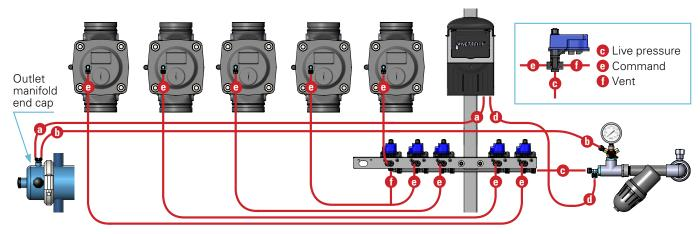
**20.** Connect the solenoids to the BackFlush controller expansion cards in sequence, from left to right. Red wire = + / black wire = common (inversing wire polarity will change NC to NO).
