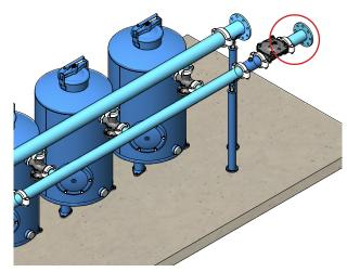
**15.** Connect the air valve to the socket on the top of the inlet manifold end-cap.
