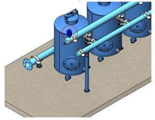
**16.** Connect the control assembly to the socket on the side of the inlet manifold end-cap.
