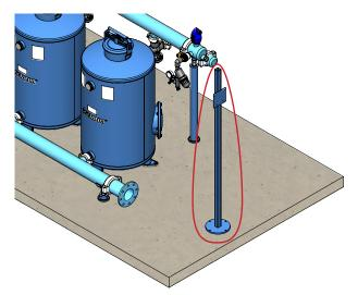
**18.** Secure the BackFlush controller and the solenoid bracket in place on the stand.
